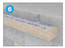
Hold the section of barrier tightly against the abutting section and secure the barrier to the substrate.
