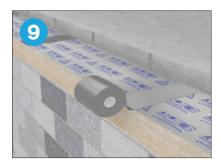
Foil tape should be applied to the upper surface in cavities 250mm to 400mm.
