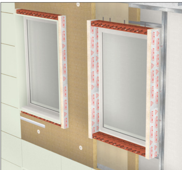
OSCB in Steel Frame / SFS construction substrate
