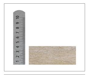
Check that the width of the strip is correct for the fire rating required.
