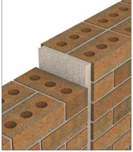
When installing Fire Stop Strip against any form of flexible wall, two fixing clips should be used per length of barrier at maximum 600mm centres.
