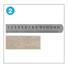
Check that the width of the strip is correct for the fire rating required.
