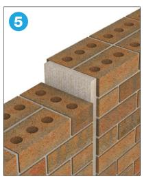
When fitting Fire Stop Strip as an expansion joint the product is push fitted into place ensuring tight butt joints between sections of barrier.
