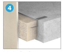
If the Fire Stop Strip is not supported by a structural element (i.e. the head of a wall) then fixing clips should be used at 600mm centres to provide support.
