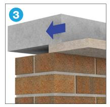
Fit the Fire Stop Strip into the void; if the substrate is rough then a temporary metal slip plate can be used.
