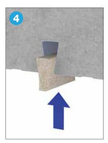
Once the Fire Stop Block is pushed through the neck of the profile it will expand to fill the void. Slide the Fire Stop Block into position over the firewall.
