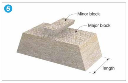
When fitting Major and Minor blocks, insert the minor profile first. A slip plate may assist in fitting the major block above rough surfaces.
