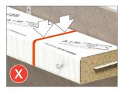
Make sure that the airspace doesn't exceed 25mm and that all of the coarse wound screws are in contact with the inside of the façade panel.
