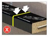
Make sure that the intumescent strip is clear to expand freely to the rear of the façade without obstruction. i.e. Vertical Cladding Rails preventing free expansion.
