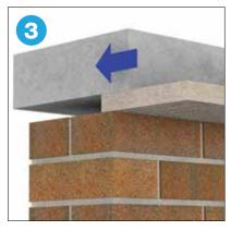
Fit the Fire Stop Strip into the void; if the substrate is rough then a temporary metal slip plate can be used.
