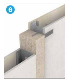
When installing Fire Stop Strip against any form of flexible wall, two fixing clips should be used per length of barrier at maximum 600mm centres.
