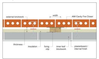
Timber Frame to Masonry outer leaf
