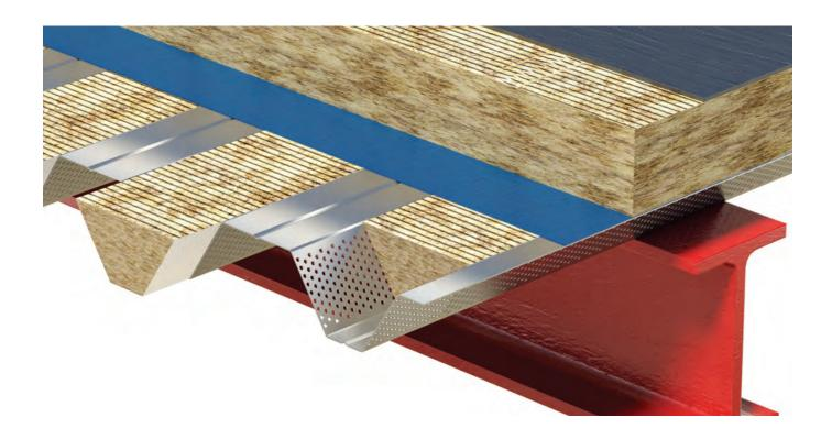
AIM Profile Trough Infills are designed to fit into the troughs of perforated metal profiles used for roof decking. They can be supplied in shapes to fit any profile and in a density to meet the requirements of the acoustic specification.
