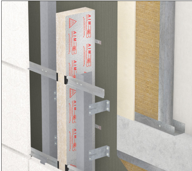
Vertical Wall Cavity Barrier intersected with a horizontal aluminium hook-on rail.
