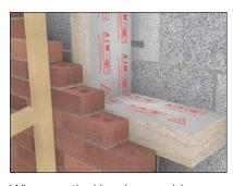
Where vertical barriers could cause "brick push" a push off post or bricklayer profile can be secured to the outside of the building as a preventative measure.
