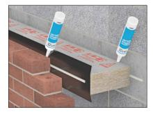
If the barrier is being installed with a DPC, apply the bead of mastic between the DPC and external leaf.
