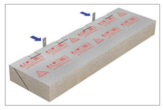
Carefully fit the Wall cavity Barrier over the fins. When fitting the barrier make sure that the cut sections doesn't snag on the sides of the fins. Secure the fixing clips back to the slab edge. Remember that all of the fixings need to be non-combustible and corrosion resistant.
