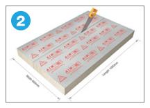
Measure the cavity depth and mark the slab. Carefully cut using an insulation saw or hand saw. Please cut in the direction of the arrows printed on the foil facing.
