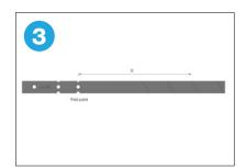
Snap the fixing clips to the correct length. Dimension X should be three quarters of the barrier's width.
