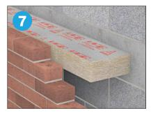
Build the brickwork up against the side of the barrier ensuring the bricks are in full and faithfull contact with the cavity barrier.
