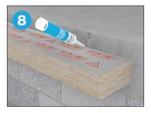
Check for any gaps between the barrier and substrates. All gaps should be fully sealed with AIM intumescent mastic.
