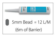
One 310ml cartridge is adequate to seal 6 linear metres of Wall Cavity Barrier against the internal and external leaf.
