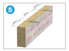
Insert two fixing clips into the barrier at 500mm centres approximately 250mm from each end.
