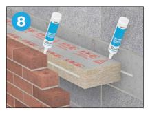
Once the mortar has cured, using an angled mastic nozzle, run a bead of mastic between the barrier and the internal and external leaf.
