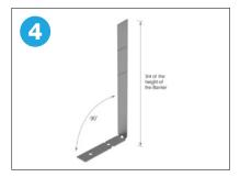
Form two fixing clips to 90° to form an L shape (three clips if the cavity is over 400mm).
