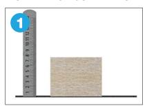
Check that the Wall Cavity Barrier is the correct thickness for the cavity. The barrier should be the same width as the cavity.
