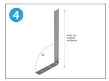
Form two fixing clips to 90° to form an L shape (3 clips if the cavity is more than 400mm).
