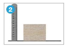
Check that the Wall Cavity Barrier is the correct thickness for the cavity. The barrier should be 5% larger than the cavity.
