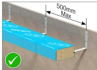
Make sure that the barrier is sitting flush back to the substrate and no gaps are present.
