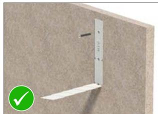
Ensure that the product is installed with the intumescent material facing towards the cladding panel. Do not apply tape over the face of the barrier.
