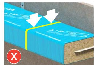
Make sure that the intumescent strip is clear to expand freely to the rear of the façade without obstruction. i.e. Vertical Cladding Rails preventing free expansion.
