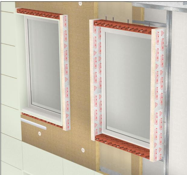
OSCB in Steel Frame / SFS construction substrate
