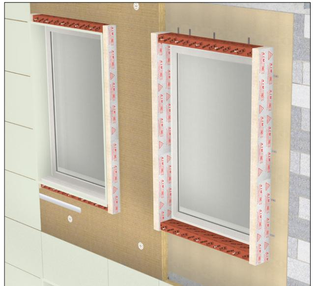
OSCB in Masonry construction substrate
