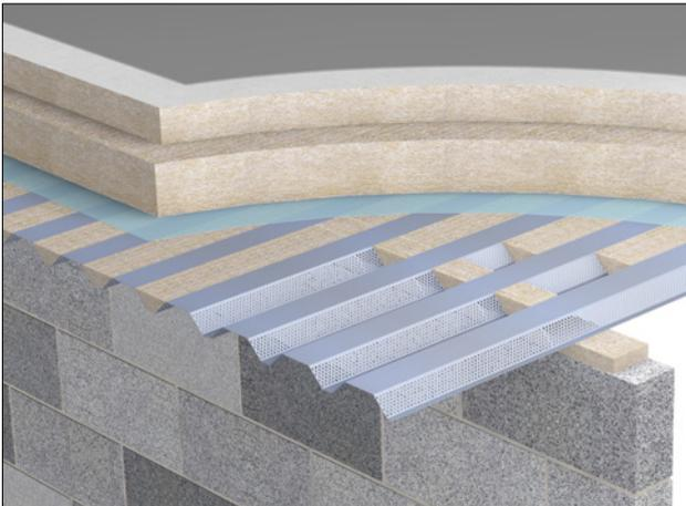
Where a fire wall is built to the underside of a perforated metal deck, AIM Fire Stop Blocks should be installed above and below deck at the line of the wall to ensure that smoke or fire is prevented from passing through the perforations in the metal work.
