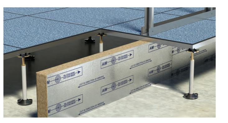
AIM Raised Access Floor Fire Barrier prevents fire from spreading under the floor void, for at least the period of fire rating specified. AIM Raised Access Floor Fire Barrier is made from high density Rockwool stone wool slab, faced with Class O foil. It is available cut to size or in slabs suitable for cutting on site.
