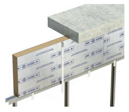
AIM Partition Head Fire Barrier is made from foil faced high density Rockwool stone wool and provides a fire barrier above fire rated metal frame partitions, fire rated timber partitions and masonry walls.
