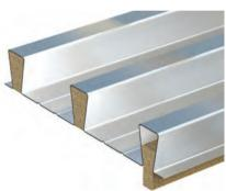
AIM Fire Stop Blocks are made from high density Rockwool stone wool. Incorporated into the building during construction, they are used to seal apertures and are permanently held in place by compression. They can also be used within metal cladding as a fire break and to protect the top flange of steel beams.
